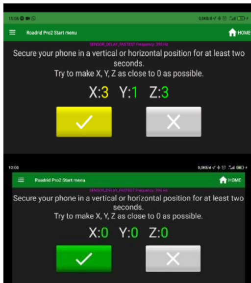
Figure 4. Roadroid calibration procedure
