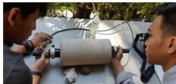
**Gambar 2.** Pengujian *UPV* Metode *Direct*
