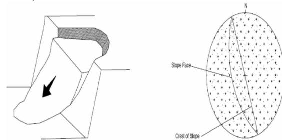
**Figure 4.** Circular failure
