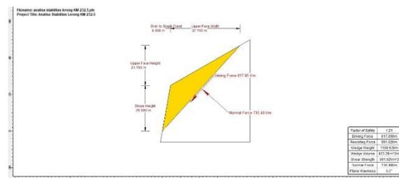
**Figure 9.** The Results of The Analysis of The Slope Stability of KM 232.5
