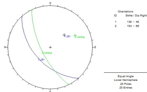
**Figure 8.** The Results of The Joint Projection Stereographic Analysis Using the Dips Software
