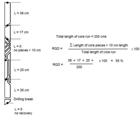
Figure 5. RQD Determination of Drill Core Samples
