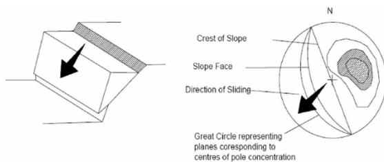
**Figure 1.** Plane failure
