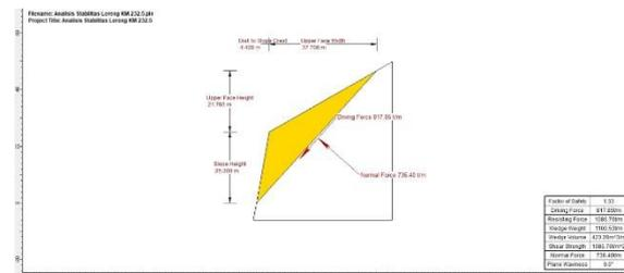
**Figure 10.** The Results of The Analysis of The Slope Stability of KM 232.5
