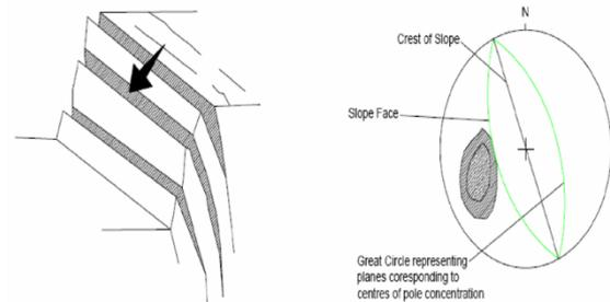
**Figure 3.** Toppling Failure
