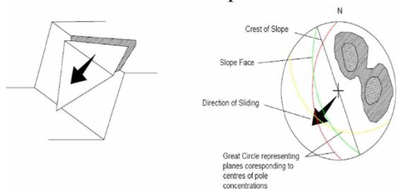
**Figure 2.** Wedge failure
