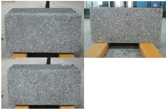
Figure 6. Onyx Concrete Panel With 4 Mm Thickness Grinding
