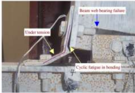
Gambar 9. Deformasi Sambungan Baut Eksperimental (Sumber: Yang, C.M., Cyclic behavior of bolted and welded beam-to-column joints )
