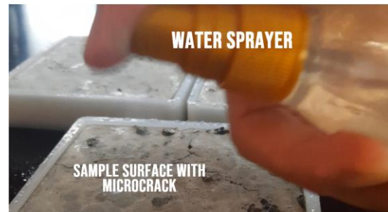
Gambar 4. Proses Spray Curing
